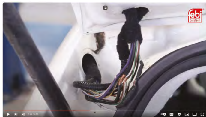
[EN] Fiat 500 tailgate wiring harness repair
